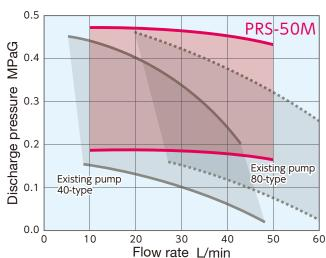
Range of flow rates corresponding to supply air pressures 0.2 to 0.5 MPaG
