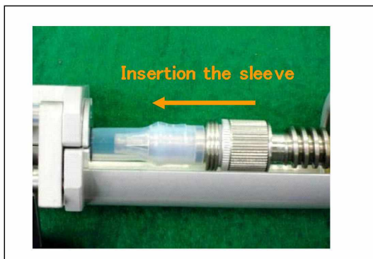
Fig. 59 – Inserting the sleeve
