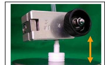
Fig. 76 - Flaring the tube
