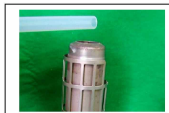
Fig. 69- Preheating the tube
